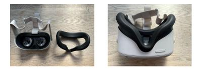
Adjust the lens IDP to, which is the distance between each eye, until you get the clearest picture. To do so gently move each lens with your thumbs to either 58mm, 63mm or 68mm.
